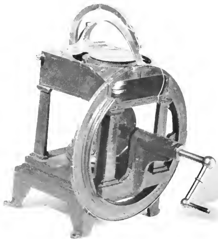
Figure 20.—BLODGETT & LEROW SEWING MACHINE, 1850, as manufactured by A. Bartholf, New York; the serial number of the machine is 19. At right, an original brass plate from the same type of machine with needle arm and presser foot and arm, serial number 119; the plate, however, does not fit the machine correctly. (Smithsonian photo 48440-D; brass plate: 48440-K.)
